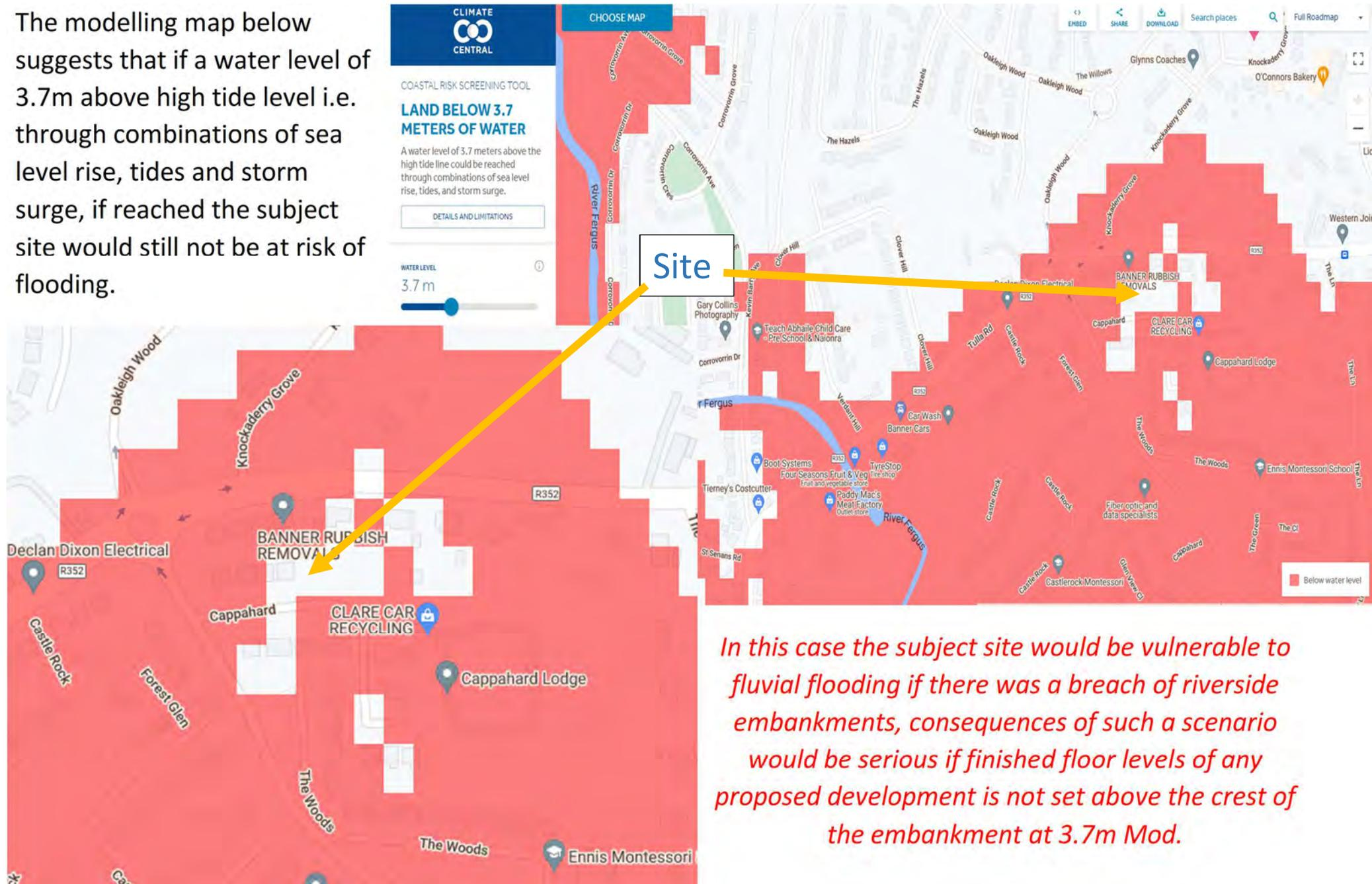
*In this case the subject site would be vulnerable to fluvial flooding if there was a breach of riverside embankments, consequences of such a scenario would be serious if finished floor levels of any proposed development is not set above the crest of the embankment at 3.7m Mod.*
